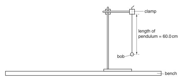
Retort stands of 60 cm or less in height may be used if the retort stand is reversed so that the pendulum hangs below the level of the bench. The base of the stand would need to be secured with a G-clamp and/or a heavy weight. Supervisors would need to warn candidates of the difference between this diagram and the set-up of their experiments.
